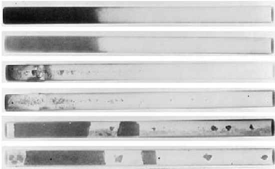
Fig. 4. X-ray photographs of the irradiated samples; from top to bottom: NaI (sample No. 1), NaI (2), \text{PbI}_2 (3), \text{PbI}_2 (4), \text{CeI}_3 (5), \text{CeI}_3 (6).
